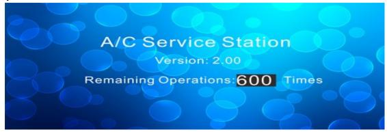
Upon 480 operations having been made, the machine displays the following message, and users can continue using the equipment meanwhile make distributor appointment
