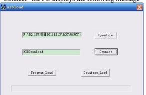
Click "Program\_load" for main program update, or click "Database\_load" for a database update, the machine displays the following:
