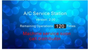
Upon 600 operations having been made, the machine will display the following message while the machine stops working. Maintenance has to be made to reset service interval time again.
