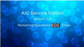
Upon 480 operations having been made, the machine displays the following message, and users can continue using the equipment meanwhile make distributor appointment
