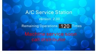
Upon 600 operations having been made, the machine will display the following message while the machine stops working. Maintenance has to be made to reset service interval time again.
