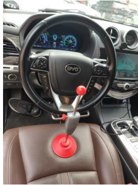
Figure 3.1-1 Steering wheel holder installation
