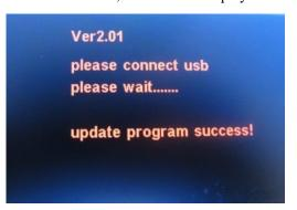
Turn off the machine and turn it on again, the machine will run the updated software.
