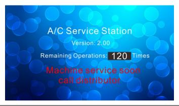
Upon 600 operations having been made, the machine will display the following message while the machine stops working. Service has to be made to reset service interval time again.
