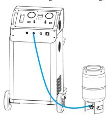
Through tank fittings, connect either HP or LP hose with external refrigerant R134a or HFO-1234yf, and turn on the machine, select "Tank fill" function, set tank fill amount to fill R134a or HFO-1234yf tank with refrigerant.
