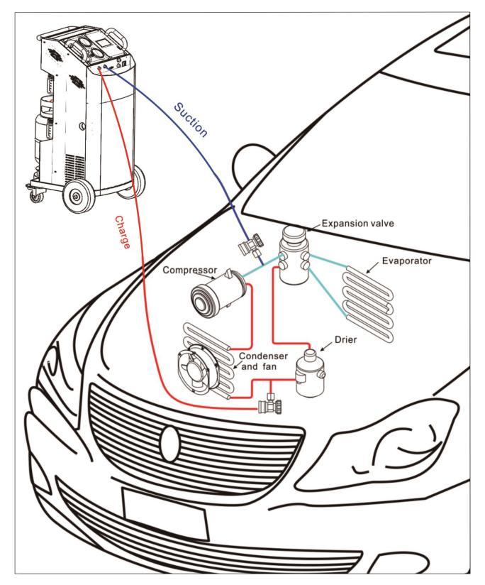
Warning: Except the situations clearly stated in the manual, during all equipment operations, please maintain the vehicle engine and A/C off, otherwise unexpected damages may be caused.
